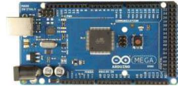
Gambar 1 Arduino Mega2560
