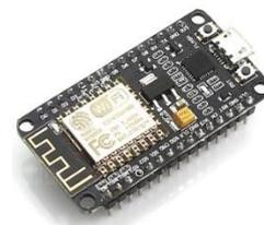
Gambar 3. NodeMCU [4]
