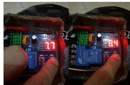
Gambar 20. set maximum voltage solar charge controller
