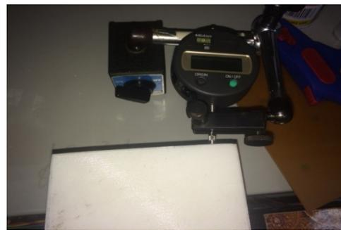
Gambar 11. Gambar Zero Dial Platform Z
