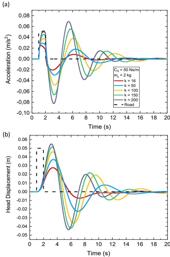
Fig. 8. Vertical (a) acceleration and (b) displacement of occupant's head with the seat-cushion stiffness coefficient variation
