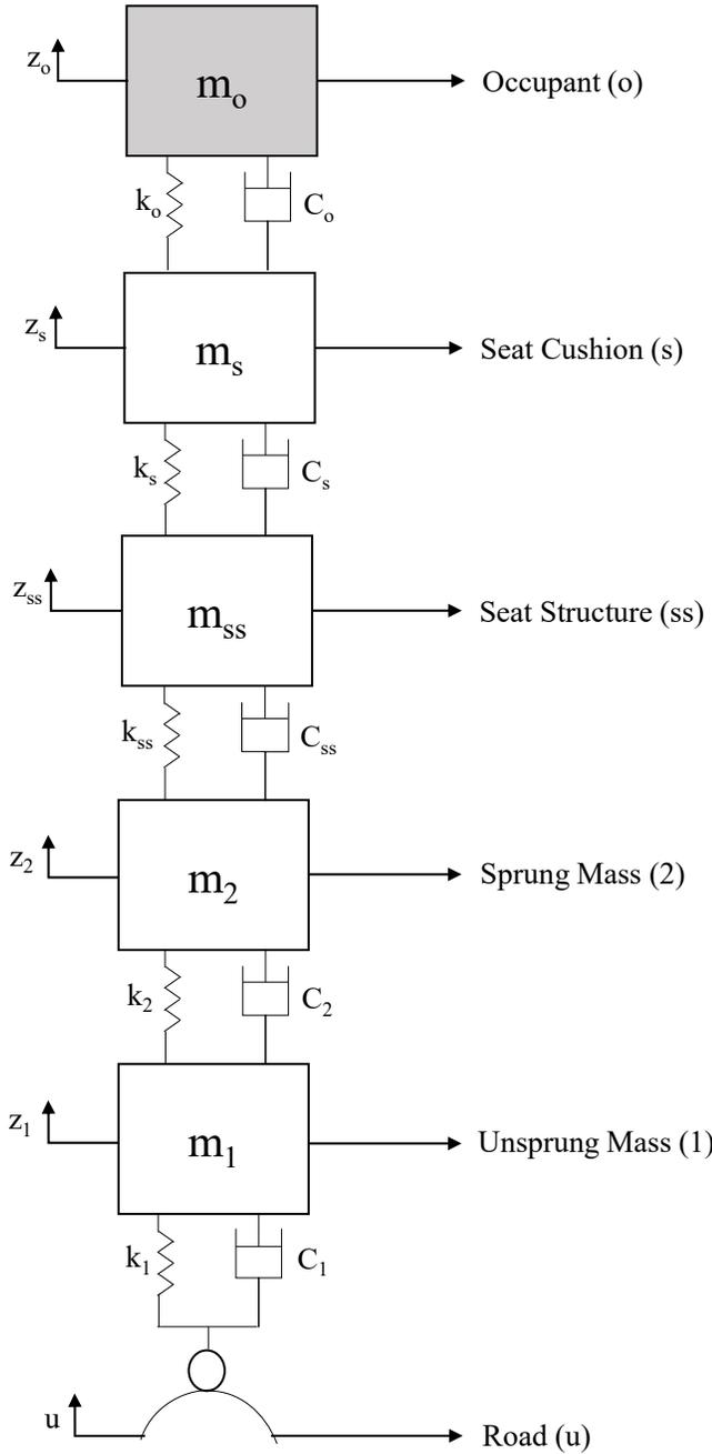
Fig. 2. Quarter-car model with seat and occupant
