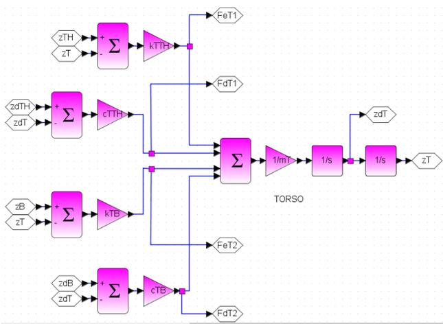
Fig. 5. Xcos-Scilab block diagram for torso modeling
