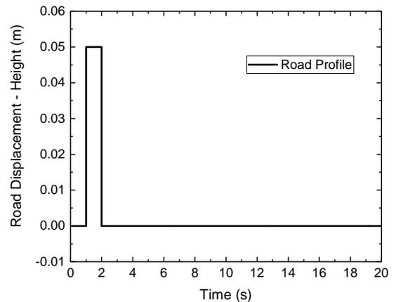
Fig. 3. Step function in respect to the time evolution as the input road profile for the simulation
