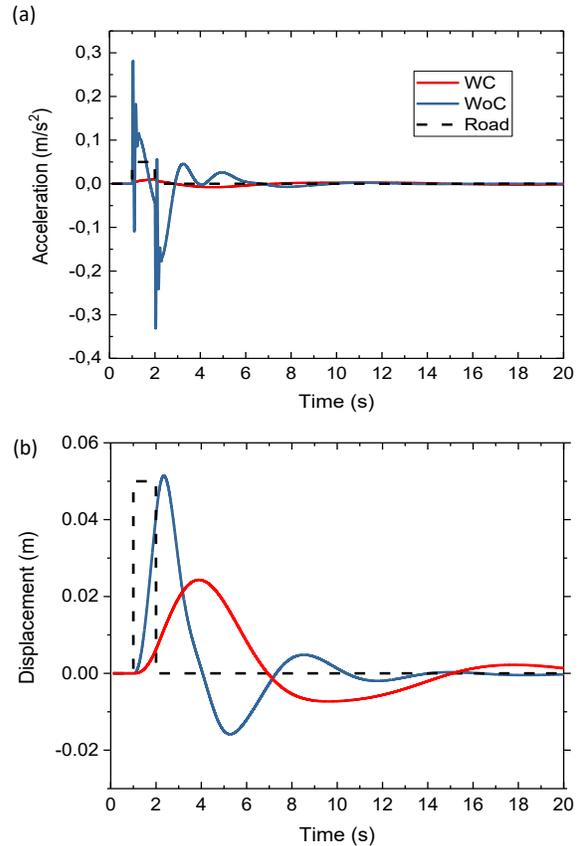
Fig. 7. Vertical (a) acceleration and (b) displacement of occupant's head with (WC) and without (WoC) a seat cushion
