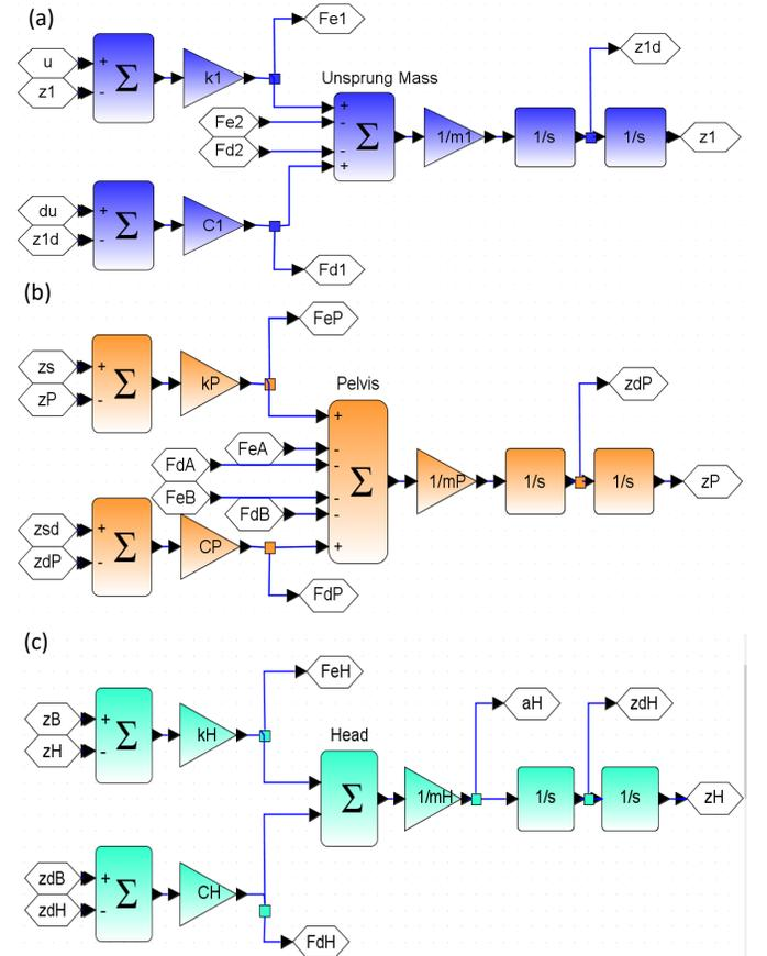
Fig. 4. Xcos-Scilab block diagram for (a) unsprung mass, (b) pelvis, and (c) head modeling
