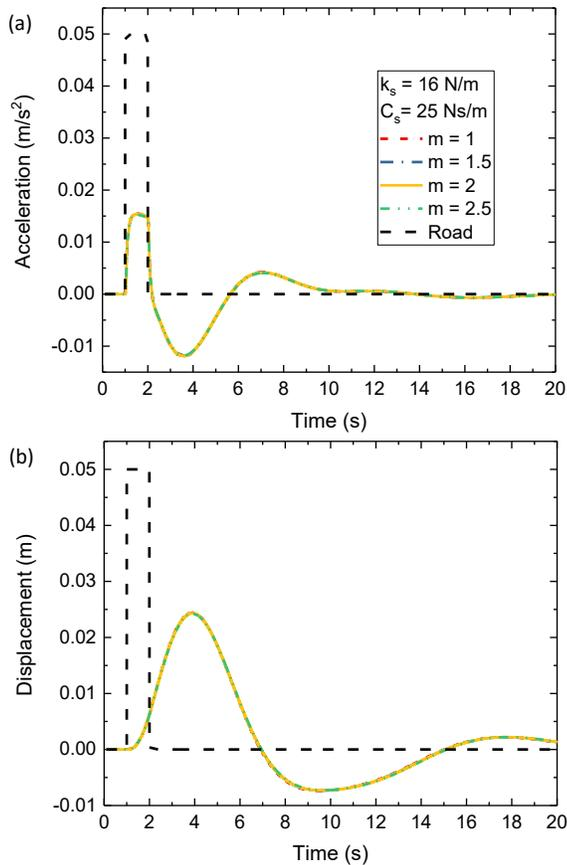
Fig. 10. Vertical (a) acceleration and (b) displacement of head with the seat-cushion mass variation
