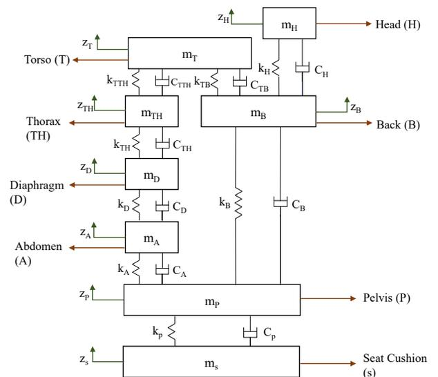
Fig. 1. 7 DoF of human model including 1 DoF of seat cushion
