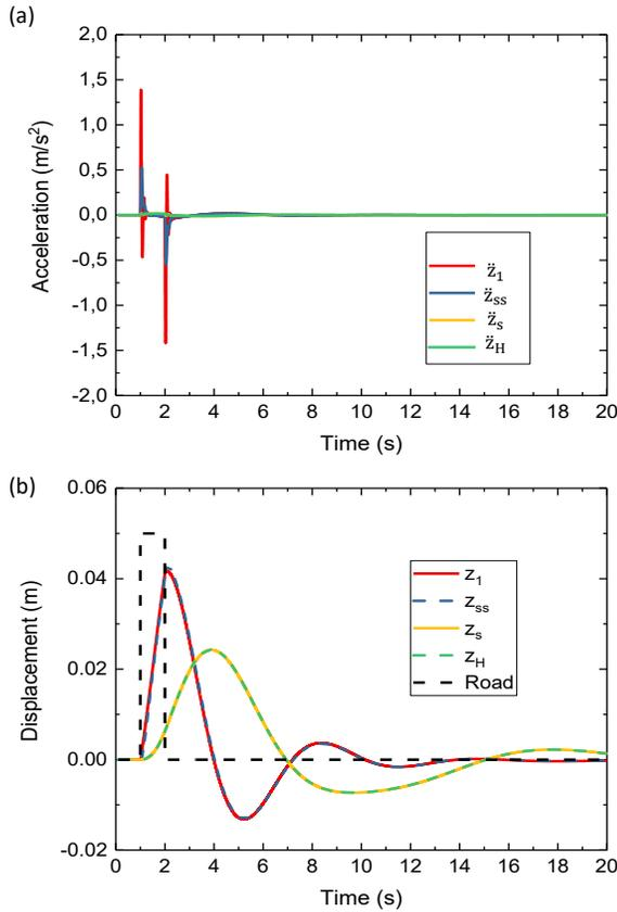
Fig. 6. Vertical (a) acceleration and (b) displacement on sprung mass ( $m_1$ ), seat structure ( $ss$ ), seat cushion ( $s$ ), and head ( $H$ )
