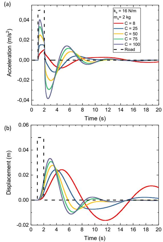
Fig. 9. Vertical (a) acceleration and (b) displacement of occupant's head with the seat-cushion damping coefficient variation
