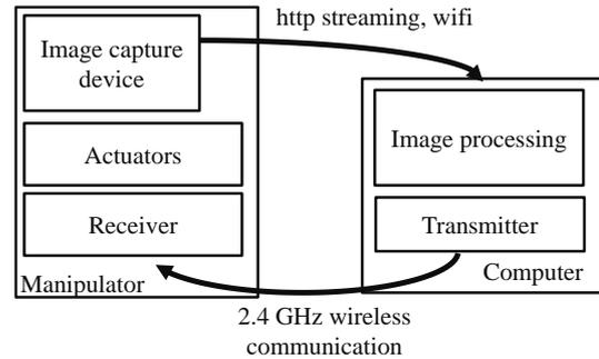
**Figure 1. Wireless visual object tracking system diagram**
