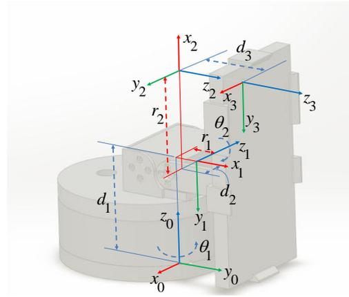
**Figure 3. Manipulator kinematics coordinate system**
