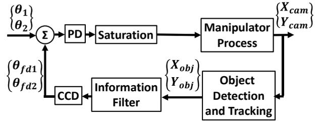
Figure 5. Visual Object Tracking Control Block Diagram
