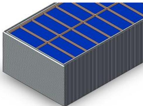
**Figure 3.** Battery enclosure design for battery pack that act as a heat sink.
