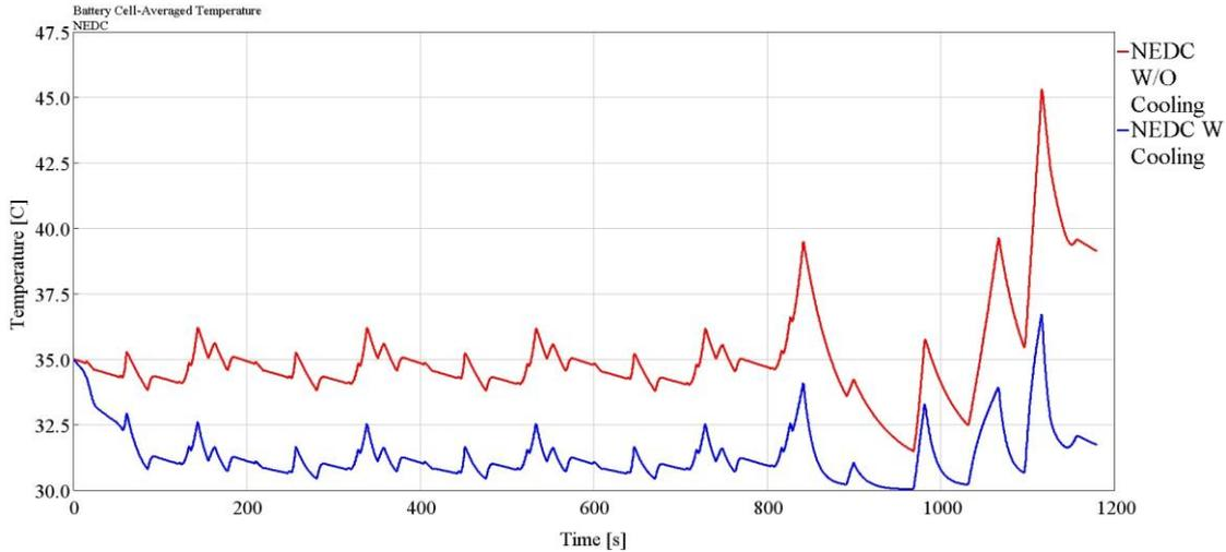
**Figure 5.** Battery temperature comparison using NEDC.
