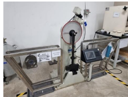
Figure 2. JB-S300 Pendulum Impact Tester
