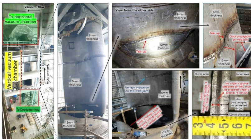
Figure 4. The Failures at Vertical Vacuum Chamber
