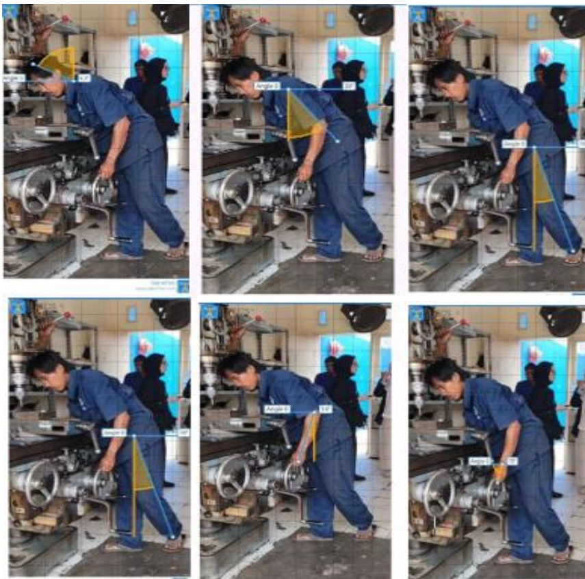
Figure 5. Milling Workstation Inclination Degree Analysis
